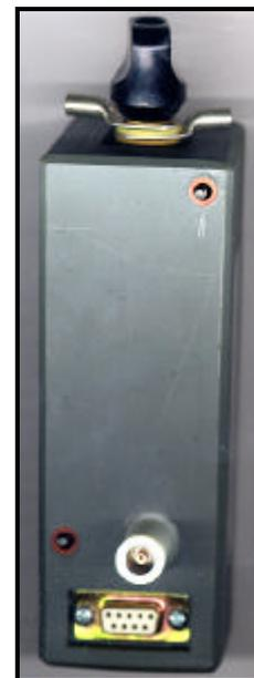
Fig. 6 : Plug-On Shunt with Triaxial Plug
